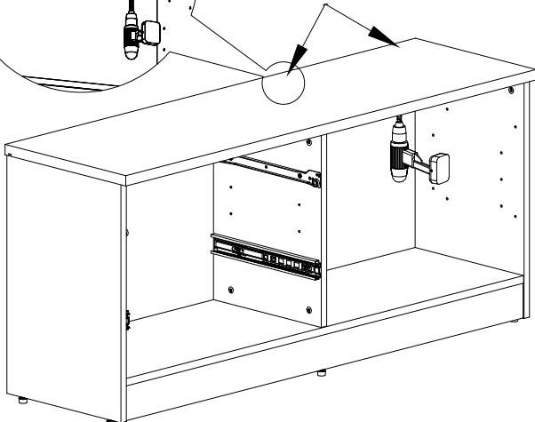
**For Right Install** finish drilling thru the pre-drilled holes on the underside of the storage return top
