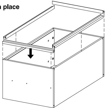
4. Attach lower storage return drawer front to box front with JCBC bolts
