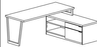
**For Left Install** finish drilling thru the pre-drilled holes on the underside of the storage return top
