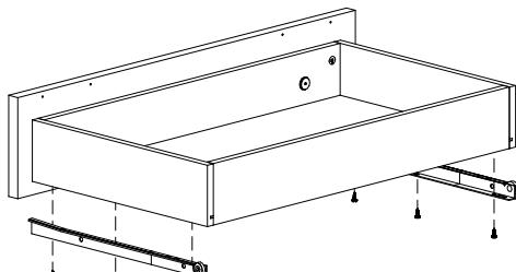
4. Align drawer slides with drawer front and secure drawer slides to drawer bottom.
