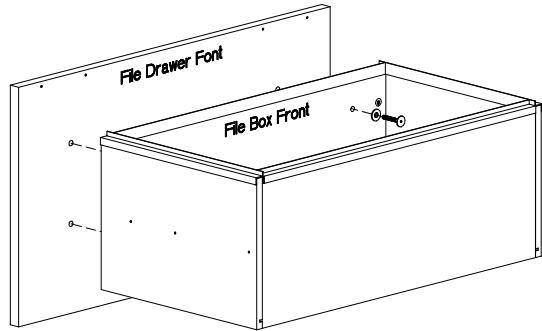
5. Align full extension drawer slide drawer component with drawer front and install on the drawer box
