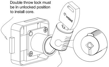
Install with key inserted in core. Align the two diamond shapes on both the bottom of the core and inside the lock housing. Tilt core at an angle and slide into housing untill core snaps in place. \*The core can be removed with the red removal key. The lock must be in the unlocked position to remove the core.
