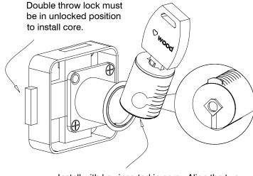
Install with key inserted in core. Align the two diamond shapes on both the bottom of the core and inside the lock housing. Tilt core at an angle and slide into housing untill core **snaps** in place.
